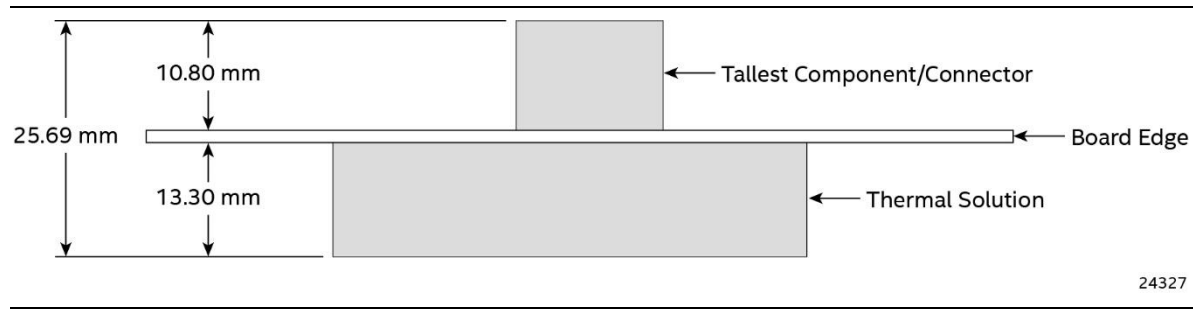
Figure 18. Board Height Dimensions
