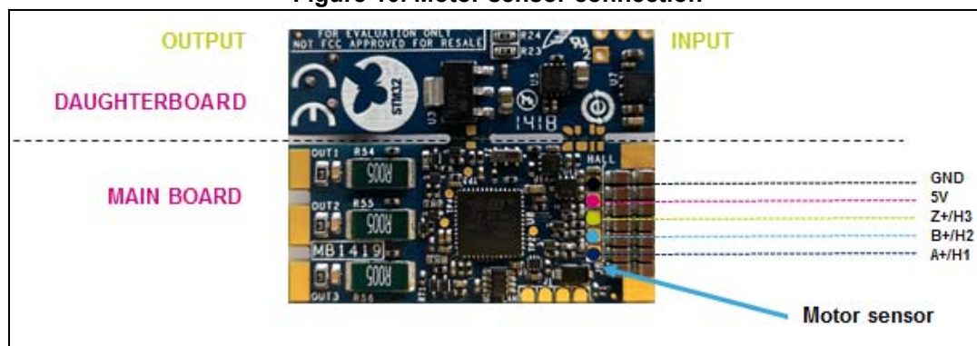
Figure 10. Motor sensor connection
