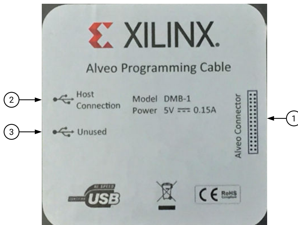
Figure 1: Alveo Programming Module Interface Locations
