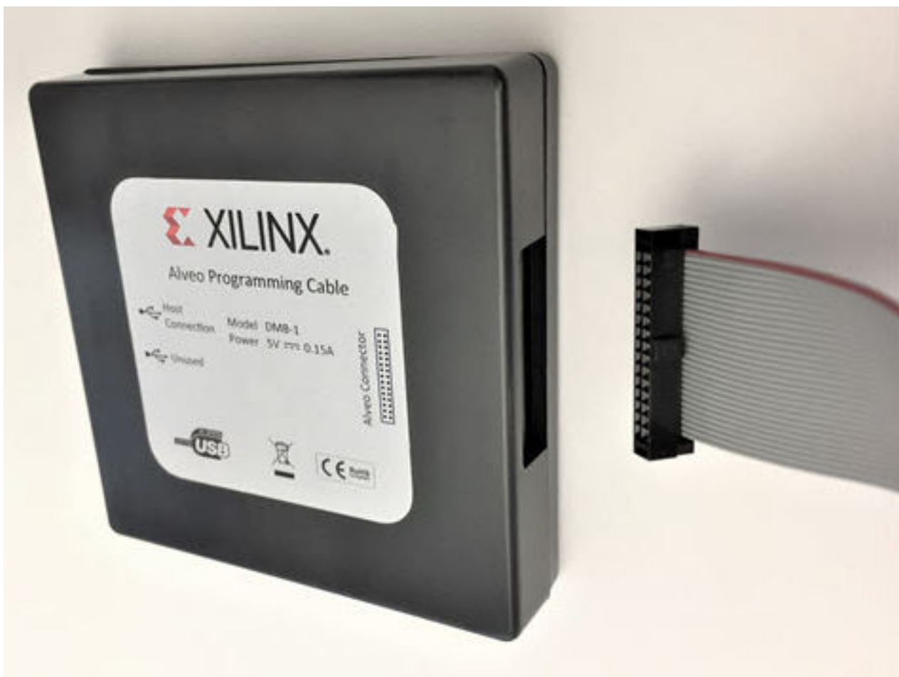
Figure 3: Connecting Ribbon Cable to Debug Connector
