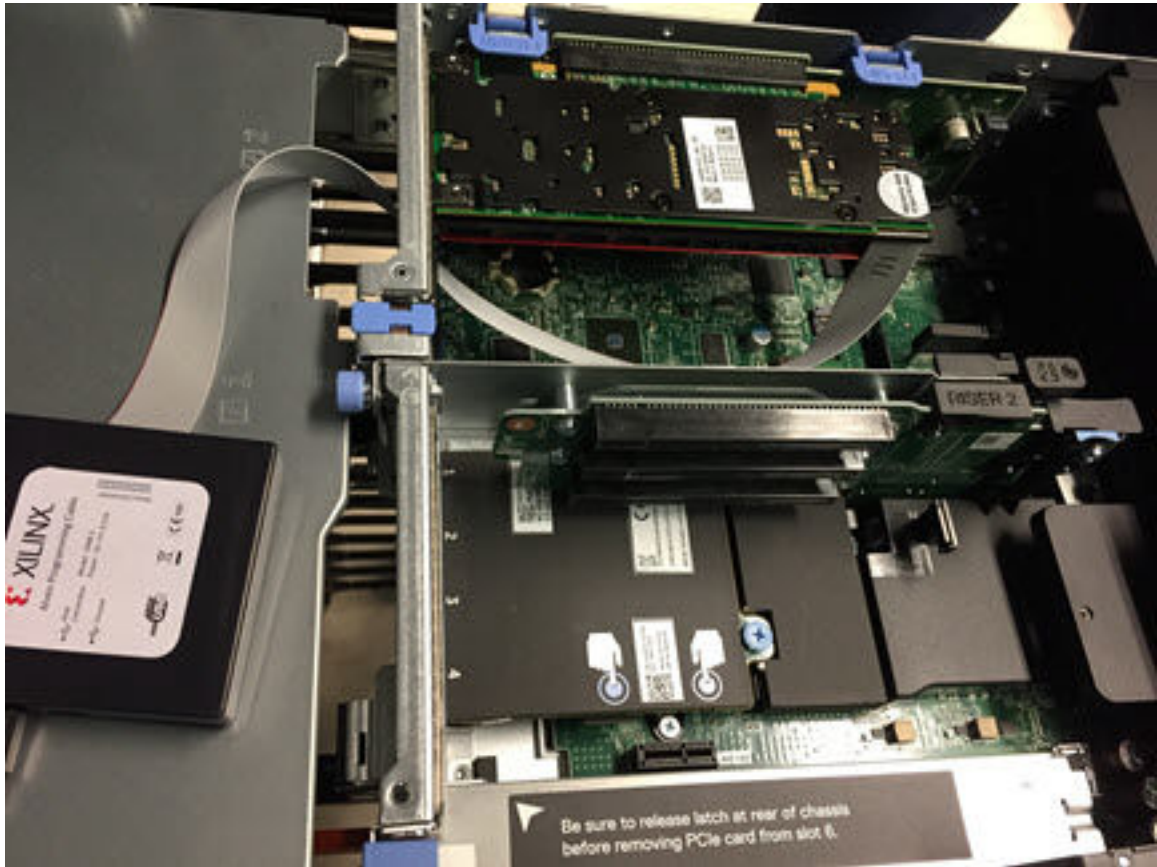
Figure 6: Installed Alveo Data Center Accelerator Card Connected to Alveo Programming Module – Side View
