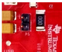
Figure 14. Current Measurement Point
