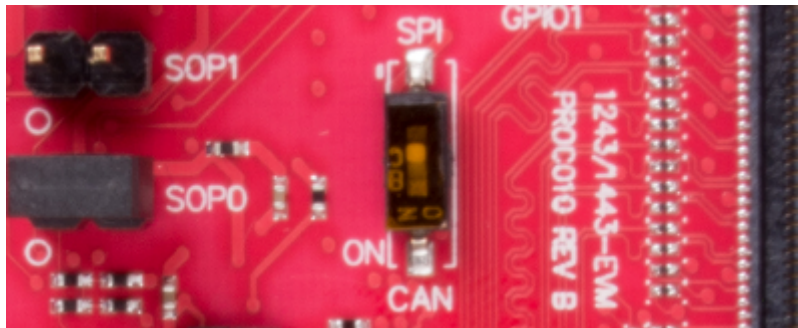
Figure 15. S1 Switch to Select Between SPI or CAN Interface
