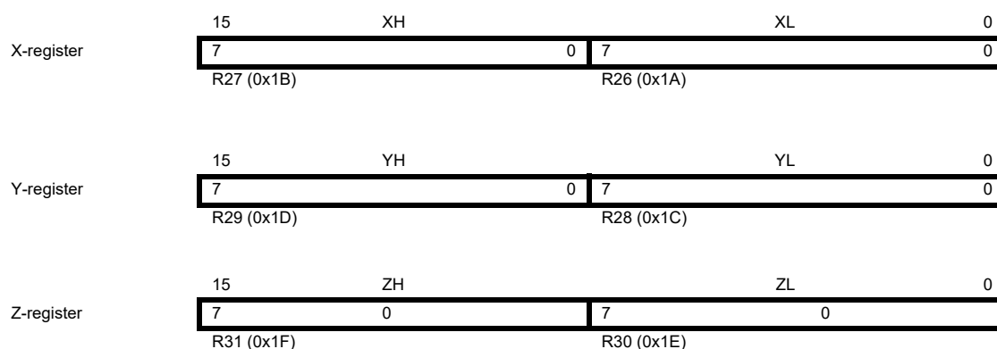
Figure 7-3. The X-, Y- and Z-Registers
