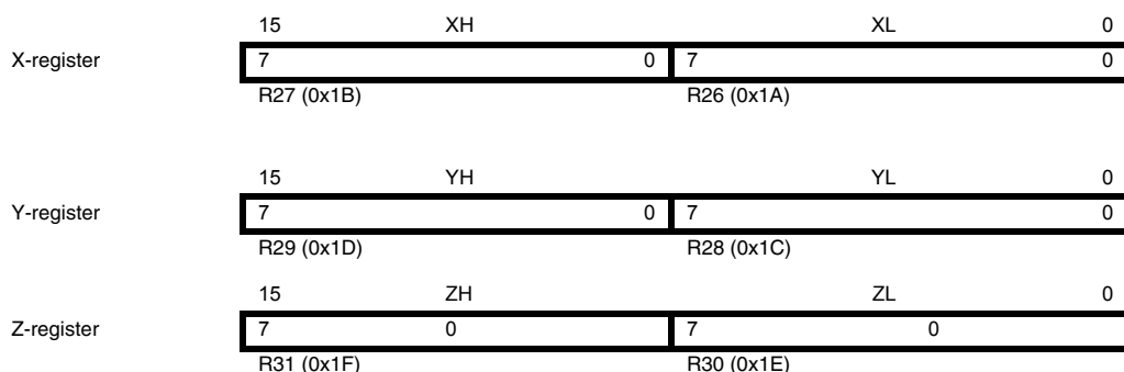
Figure 6-3. The X-, Y-, and Z-registers
