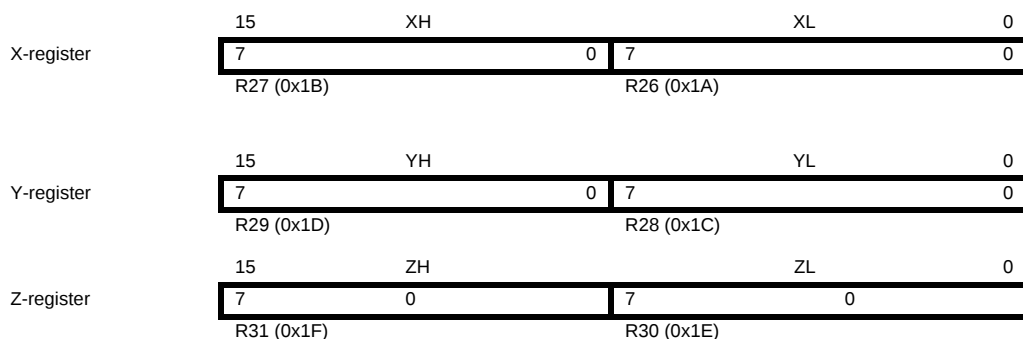
Figure 6-3. The X-, Y-, and Z-registers
