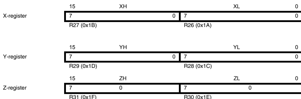
Figure 6-3. The X-, Y-, and Z-registers
