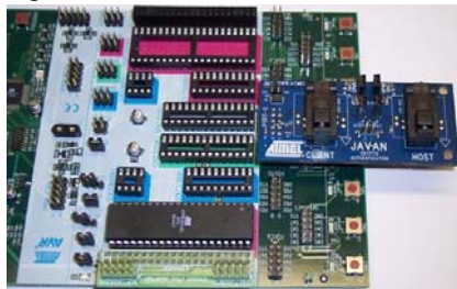
Figure 18. AT88CK109BK3 Mounted to the STK500
