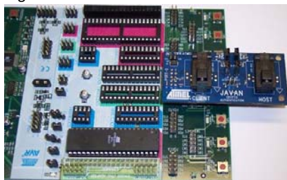
Figure 18. AT88CK109BK3 Mounted to the STK500
