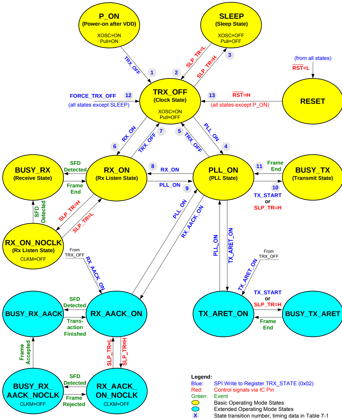
Figure 7-5. Extended Operating Mode State Diagram
