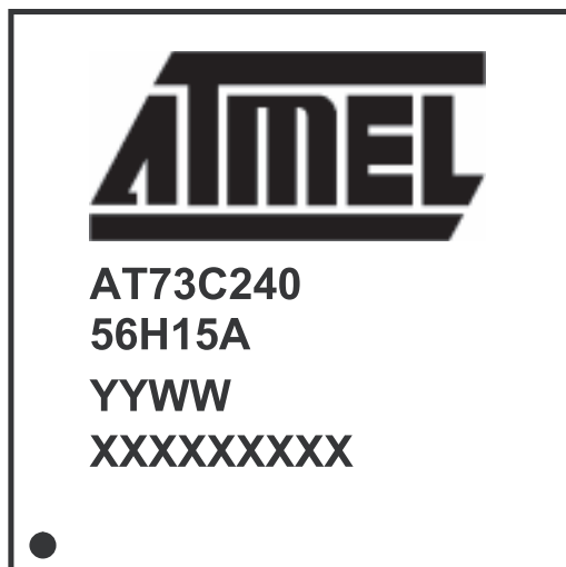
Figure 15-2. Package Drawing with Pin 1 and Marking for R-QFN032_H package
