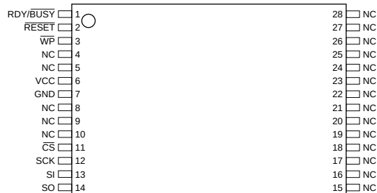
TSOP Top View Type 1
