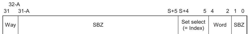
Figure 4-3 ARM926EJ-S cache Set/Way/Word format
