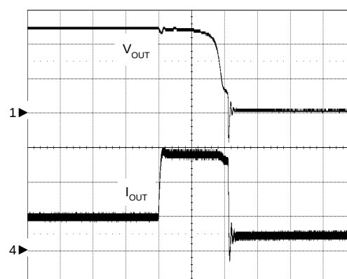
Over Current Protection
