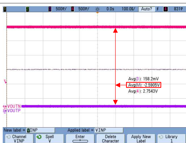
Figure 51. Typical Failsafe Output of the AMC1302-Q1
