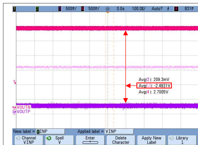
Figure 50. Typical Negative Clipping Output of the AMC1302-Q1
