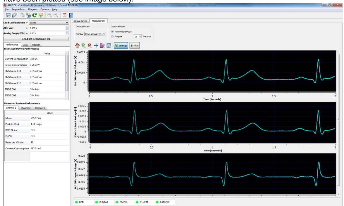
Figure 12: ECG Plot for 3-channels (5-lead) measurement
