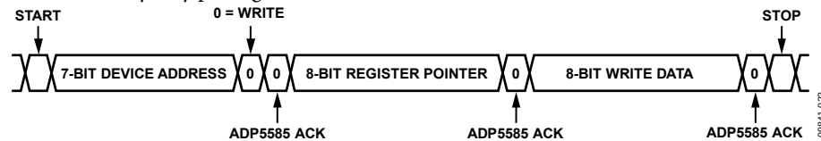
Figure 23. I 2 C Single Byte Write Sequence
