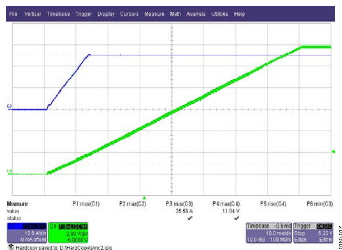
Figure 18. Startup at 385 V DC, 25 A Load (1 A/μs Slew Rate) Green Trace: Output Voltage, 2 V/div, 10 ms/div Blue Trace: Load Current, 10 A/div, 10 ms/div
