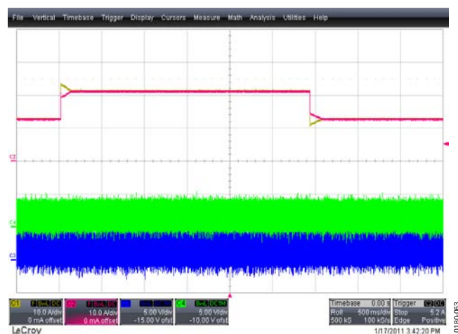
Figure 64. Digital Current Sharing with Load Step of 25 A, 42 A, 25 A Red and Yellow Traces: Output Currents of PSU1 and PSU2, 10 A/div, 500 ms/div Green and Blue Traces: SHAREo Pins of PSU1 and PSU2, 5 V/div, 20 ms/div
