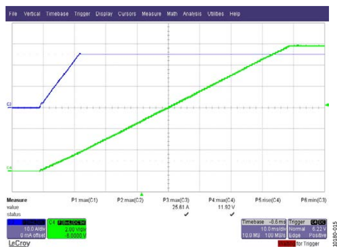
Figure 16. Startup at 350 V DC, 25 A Load (1 A/μs Slew Rate) Green Trace: Output Voltage, 2 V/div, 10 ms/div Blue Trace: Load Current, 10 A/div, 10 ms/div
