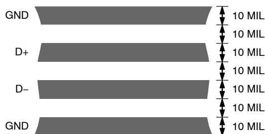
Figure 18. Typical Arrangement of Signal Tracks
