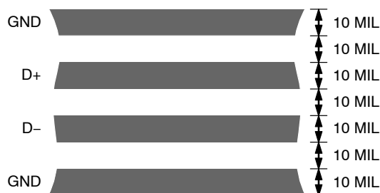
Figure 18. Typical Arrangement of Signal Tracks
