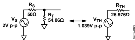
Figure 107. Thevenin Equivalent Circuit
