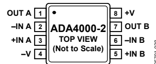
Figure 4. 8-Lead MSOP (RM-8)
