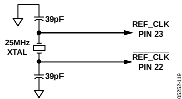
Figure 35. Crystal Input Configuration
