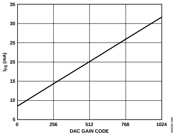
Figure 63. I_{\text{FS}} vs. DAC Gain Code
