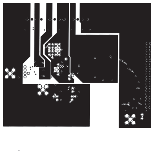
Figure 16. PCB Power Layers—Layers 3 and 4
