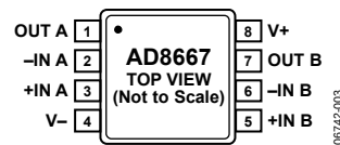
Figure 3. 8-Lead MSOP (RM-8), 8-Lead SOIC (R-8)
