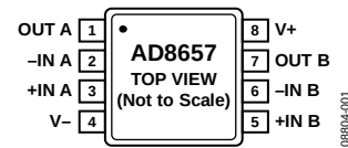
Figure 1. AD8657 Pin Configuration, 8-Lead MSOP
