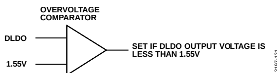
Figure 125. Digital LDO Monitor
