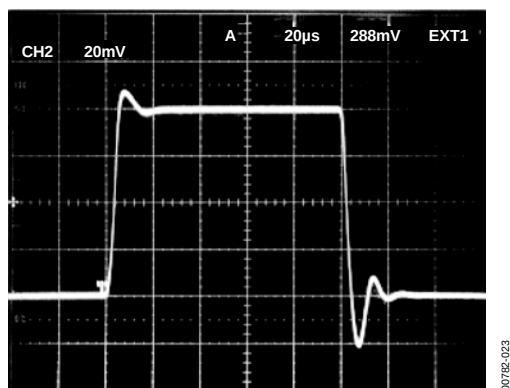
Figure 25. Small Signal Pulse Response, G = +5 , R_L = 20 \text{ k}\Omega , C_L = 50 \text{ pF}
