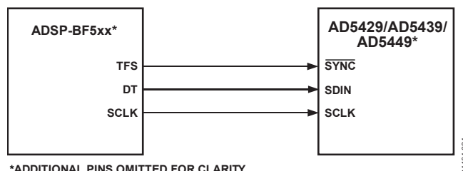
Figure 51. ADSP-BF5xx SPORT-to-AD5429/AD5439/AD5449 Interface
