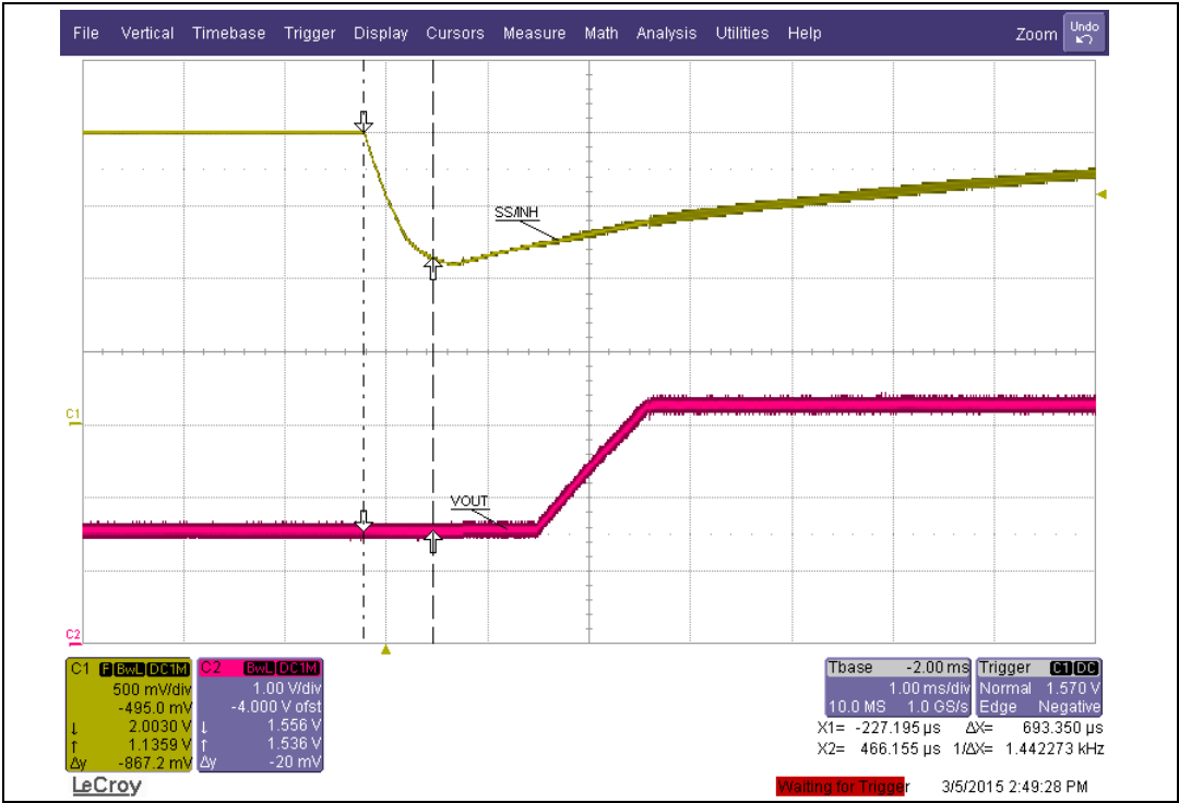
Figure 9. External soft-start after UVLO or thermal shutdown
