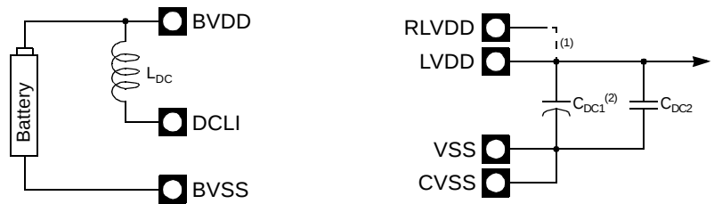
Figure 135. Battery DC-DC Connection
