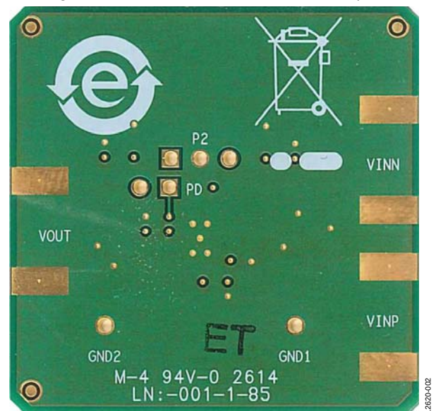
Figure 2. SO8 SINGLE AMP Evaluation Board, Secondary Side
