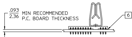
RECOMMENDED P.C. BOARD INSTALLATION SCALE 1:1
