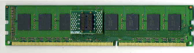
BGA Interposer probing solution for DDR2/DDR3
